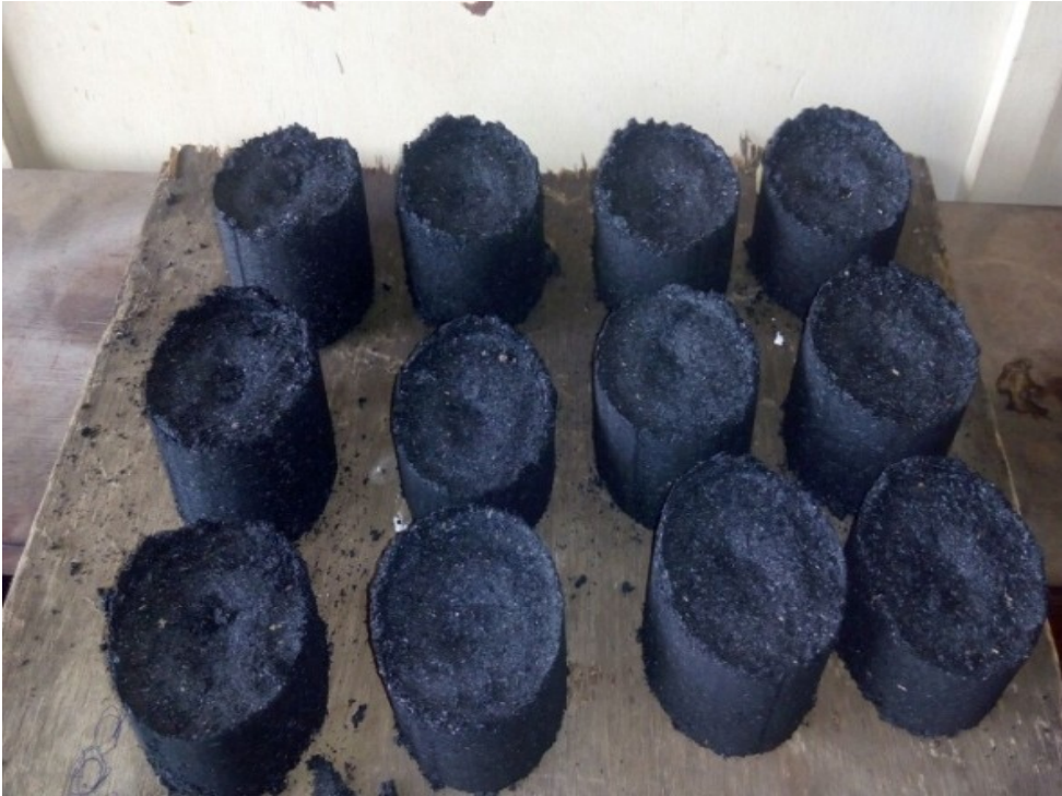
Plate 1: Charcoal briquettes produced from Gmelina arborea
